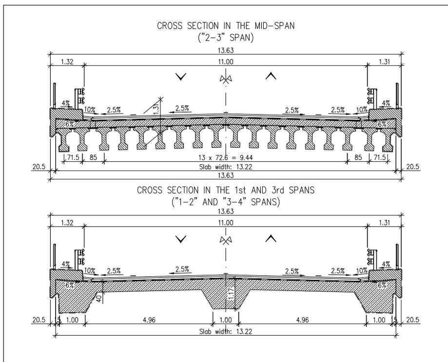
Fig. 17: Cross-section of the Perkáta bridge
