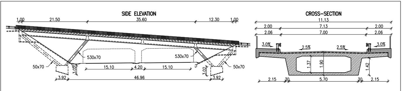
**Fig. 7:** Design of bridge over M0 motorway under earth-road and footpath
