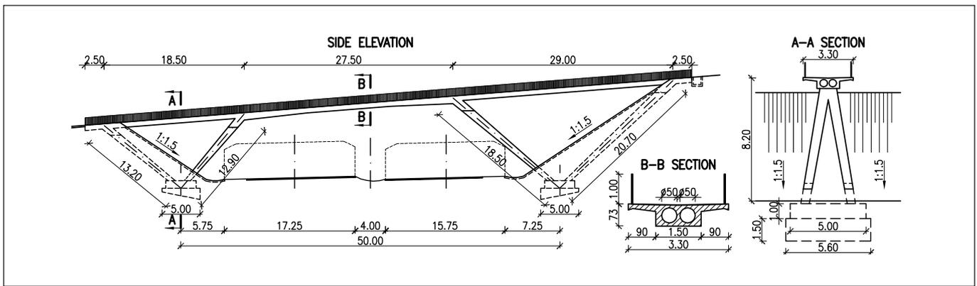
Fig. 3: Drawing of the footbridge over M7 motorway near Velence
