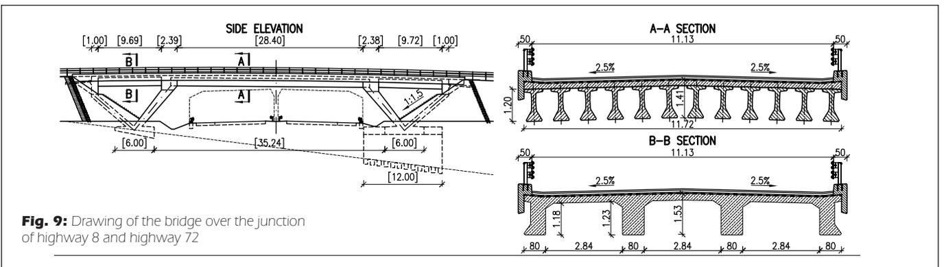
**Fig. 9:** Drawing of the bridge over the junction of highway 8 and highway 72
